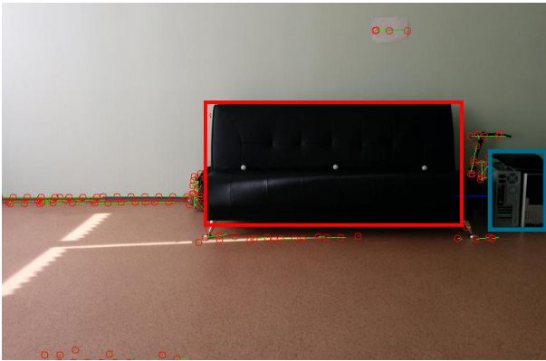
Fig. 5. Example of objects excluding by CNN: the black sofa (in red rectangular) and the PC blocks (in blue rectangular).
