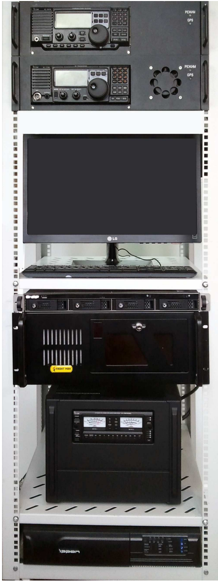
Figure 2. A single-position version of an automated two-channel EIS.
