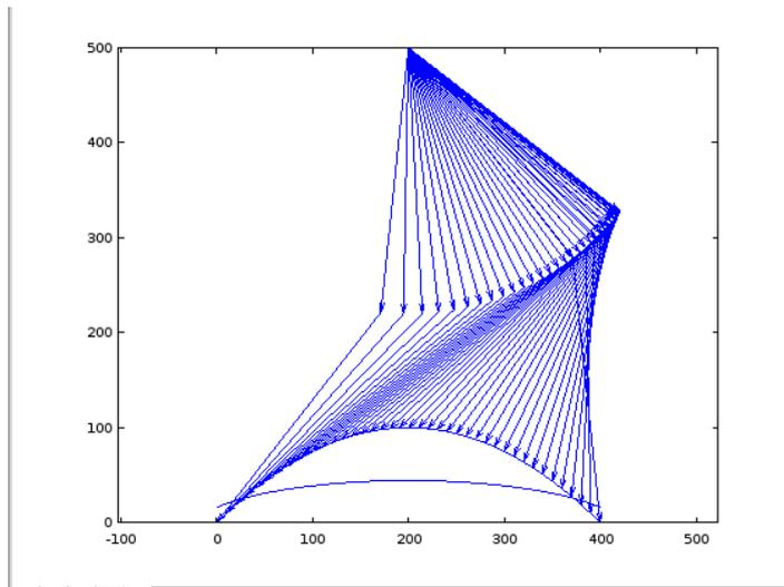
Fig.2. Moving not-supported leg on a parabolic trajectory.
