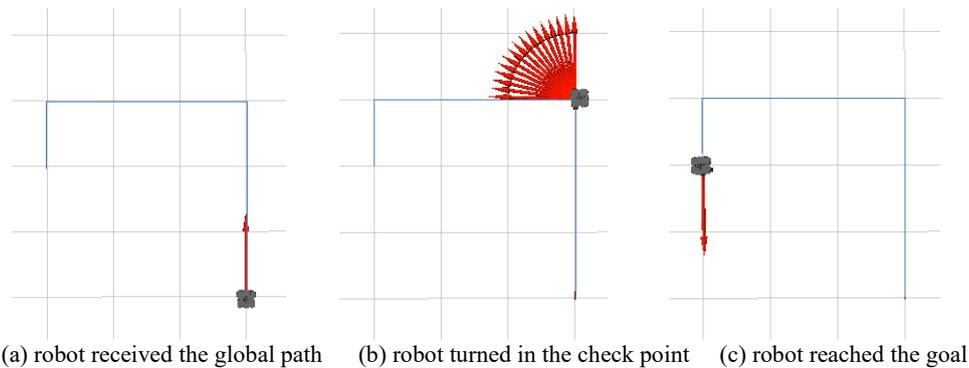
Fig. 7. The robot executed the path following task which was published from remote server. © The 2019 International Conference on Artificial Life and Robotics (ICAROB2019), Jan. 10-13, B-Con Plaza, Beppu, Oita, Japan
