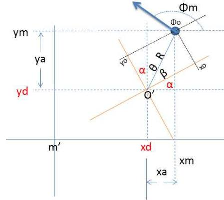
Fig. 4. Coordinate Transform between world (map) and odometry.
