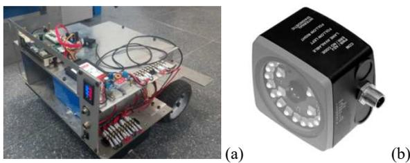
Fig. 1. (a) a differential wheeled robot platform equipped with an industrial PC (b) the optical reading head (PGV 100 serial) for barcode tag identification
