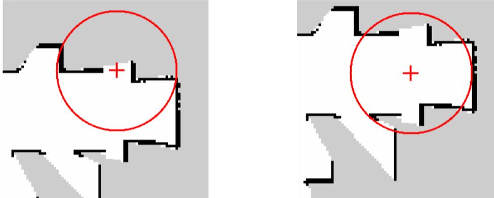
**Figure 3.** The red cross marks an observing point (a robot position) and the red circle represents a robot sensor range. Greedy approach observing point is located at the free space frontier (left) and our approach observing point is located in the free space with several unknown regions within sensory range (right).
