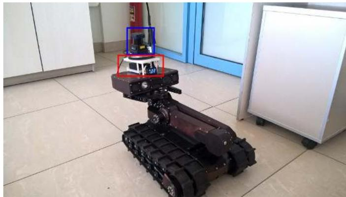
**Figure 7.** Servosila Engineer robot at starting position with LRF (encapsulated in the blue rectangle) installed on a stand with a voltage regulator and a voltage indicator (encapsulated in the red rectangle). The laser beam is parallel to the floor surface.
