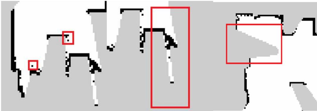
**Figure 1.** The maps are constructed by Servosila Engineer robot during an experiment. Mapping artifacts are encapsulated in the red rectangles: impulse noises (left), a processing error (center), a space between distinct laser scans (right).
