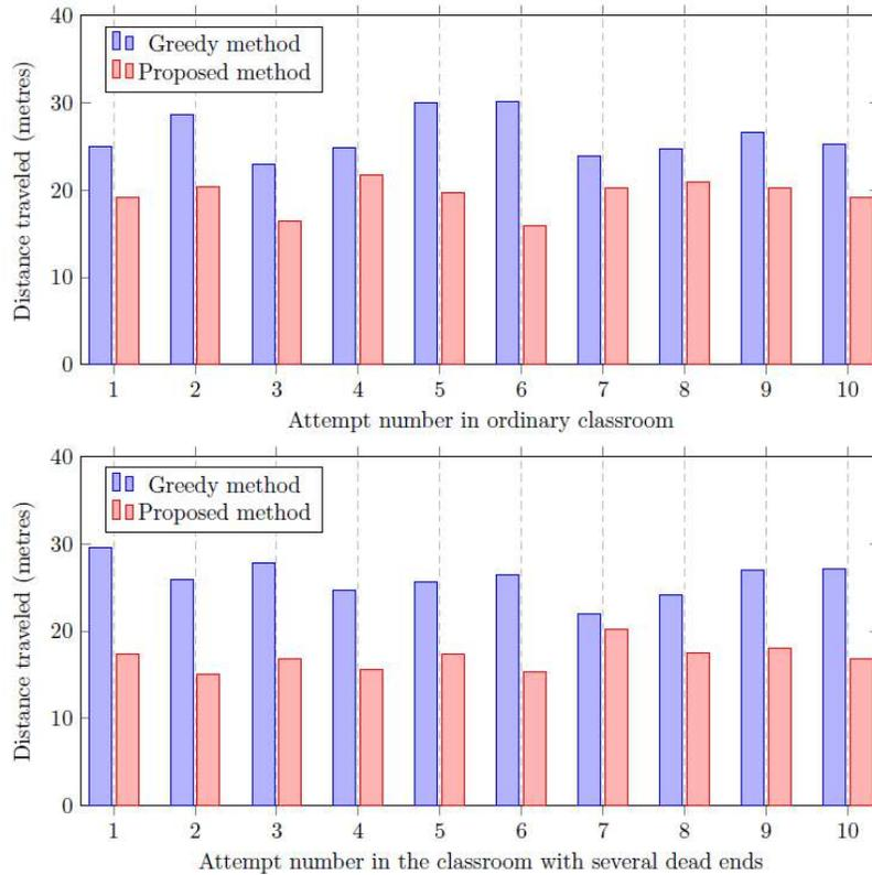
**Figure 10.** Distance travelled in the experiments: the ordinary classroom arrangement (top) and the classroom arrangement with several dead ends (bottom).
