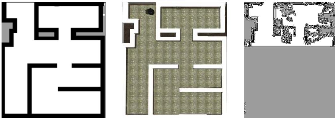
Figure 5. Automatic heightmap creation tool demonstration. Original map (left), and a 3D Gazebo simulation environment that was created using the original map (center). The map was used in simulations as an input for a robot (right).
