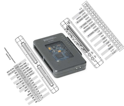
Fig. 2 MyRio-1900 control box
