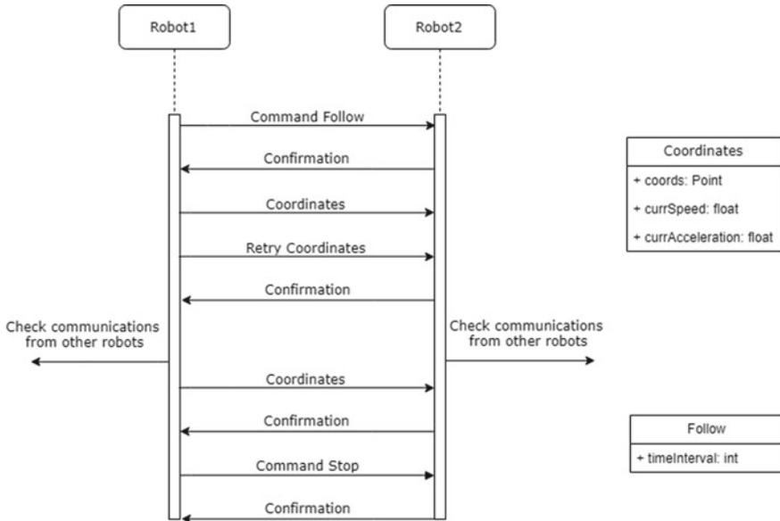
Fig. 2.4 Diagram for “Follow” command protocol
