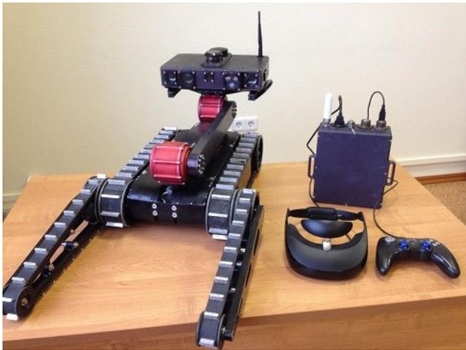
Figure 1. Tracked robot "Engineer"
