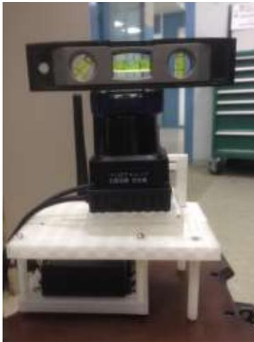
Figure 3. Hokuyo laser on a stand. Laser is parallel to the surface of the floor.
