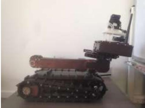
Figure 2. Servosila Engineer crawler-type robot with a Hokuyo UTM-30LX-EW LRF mounted on its top.
