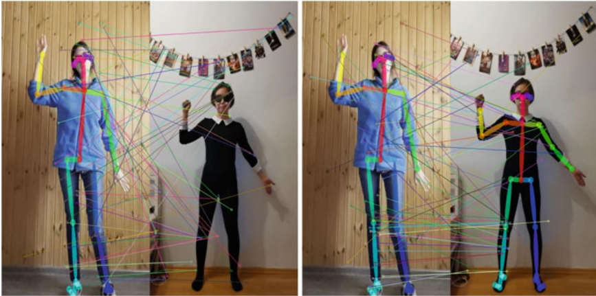
Fig. 7 A direct matching of postures without skeleton use (the upper row, 106 matches) and a skeleton-based matching (the bottom row, 101 matches)
