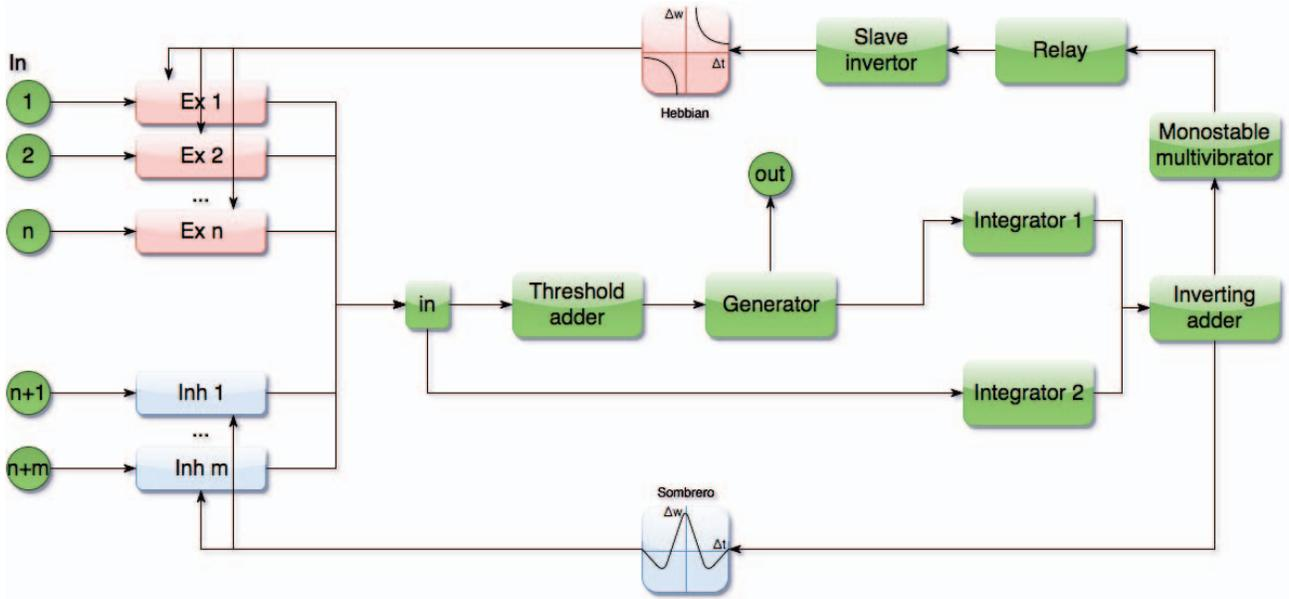
Figure 1. The block diagram of memristive artificial neuron. Inputs are depicted as green circles 1, ..n, ..n + m, “Ex..” and “Inh..” are excitatory and inhibitory memristive elements “in” is meta-element that represents all integrated inputs, “out” the output of the device
