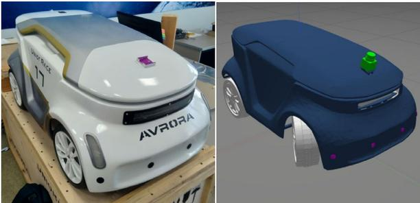
Fig.2. Avrora Robotics Junior robot (left image) and its model in Gazebo (right image).
