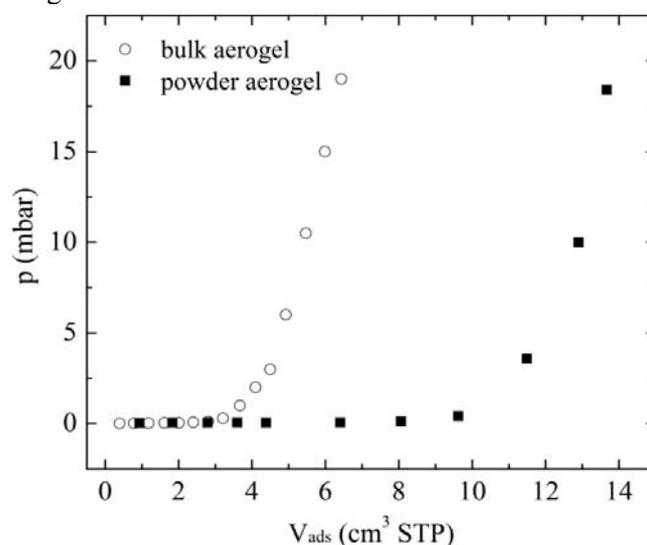
**Figure 3.** Adsorption isotherms of  $^3\text{He}$  in bulk and powder aerogel samples at temperature 4.2 K.
