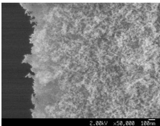
**Figure 1.** TEM of silica aerogel with filamentary structure
