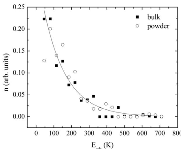
**Figure 8.** Binding energy distributions of  $^3\text{He}$  in two types of aerogel
