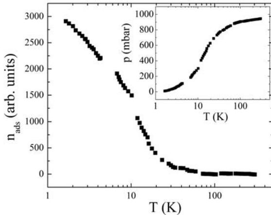
**Figure 6.** Temperature dependence of  $^3\text{He}$  amount adsorbed in powder aerogel in case of  $V(^3\text{He}) = 24 \text{ cm}^3 \text{ STP}$ . On insert shown the  $p(T)$  dependence.
