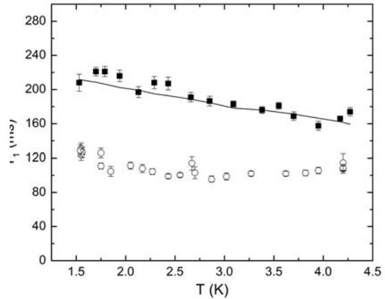
**Figure 7.** The temperature dependences of  $^3\text{He}$  longitudinal relaxation time  $T_1$  in powder aerogel:  $\circ$  –  $V(^3\text{He}) = 12 \text{ cm}^3 \text{ STP}$ ,  $\blacksquare$  –  $V(^3\text{He}) = 24 \text{ cm}^3$
