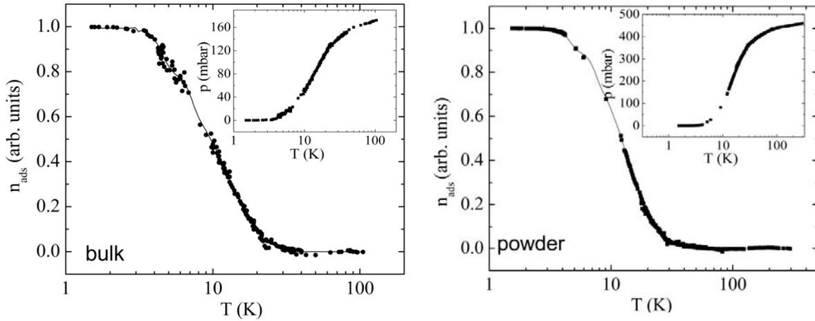
**Figure 5.** Temperature dependences of  $^3\text{He}$  amount adsorbed in aerogel: dots – experimental data ( $V(^3\text{He}) = 4.7 \text{ cm}^3 \text{ STP}$  -experiment with bulk aerogel,  $V(^3\text{He}) = 12 \text{ cm}^3 \text{ STP}$ - experiment with powder aerogel), lines – Langmuir model (see text). On inserts shown the  $p(T)$  dependences.
