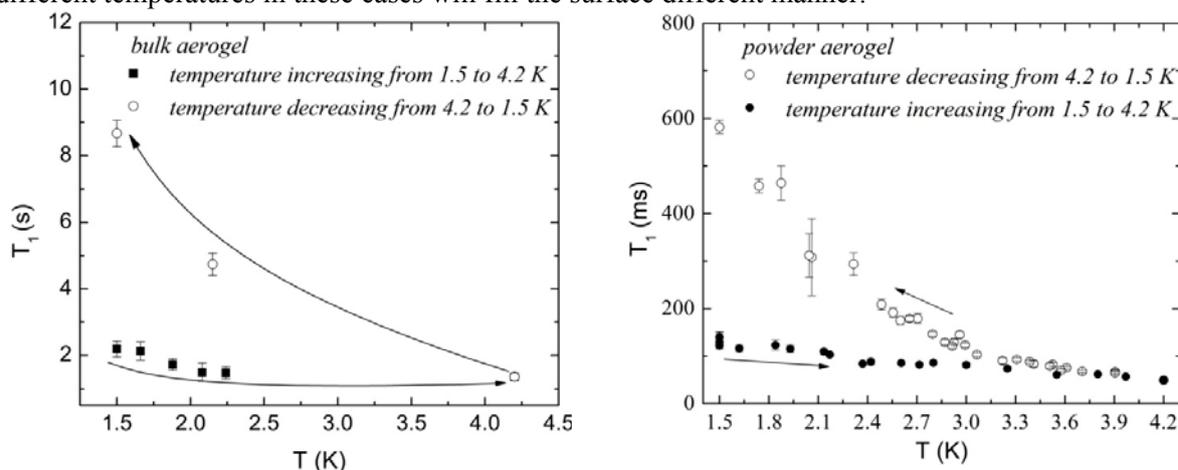
**Figure 4.** The temperature dependences of  $^3\text{He}$  nuclear longitudinal relaxation time  $T_1$  for incomplete adsorbed layer. The adsorbed layer was prepared at two different temperatures (1.5 K and 4.2 K).
