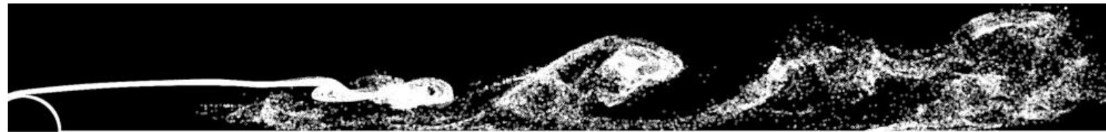
Transition to turbulence and intensification of heat exchange past a rib
