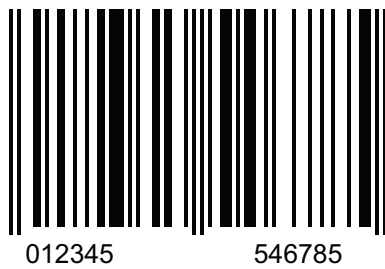
Fig. 3: UPC - UPC-A Code with the information “01234554678” of the size SC5 (see Table 8)
