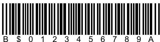
Fig. 10: Codabar with B as start and A as stop bit.
