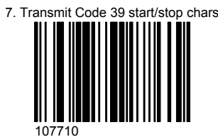
Fig. 37: Transmit Code 39 Start / Stop Character
