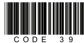
Fig. 11: Code 39 Symbol with the Information “CODE 39”
