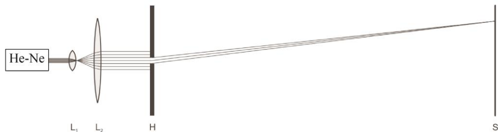
Fig. 4. Experimental setup for observing diffraction at a slit on the translucent screen. L_1 and L_2 are lenses with the focal length f = +5 mm and f = +50 mm. H - diaphragm with 3 fixed width slits which is inserted in a holder with spring clips, S - translucent screen.
