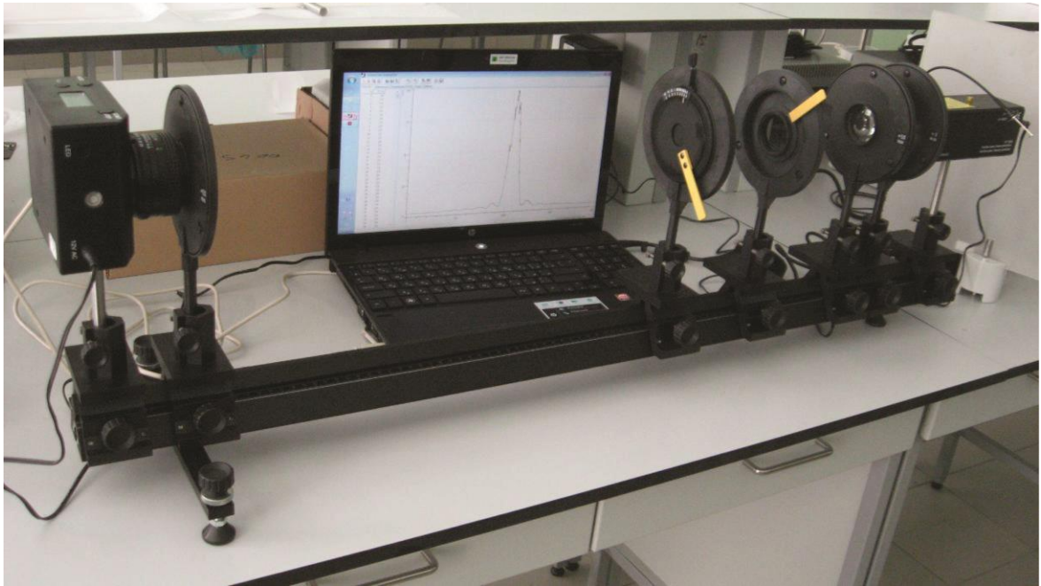
Fig.2. Experimental setup for observing diffraction at a slit by VideoCom system.
