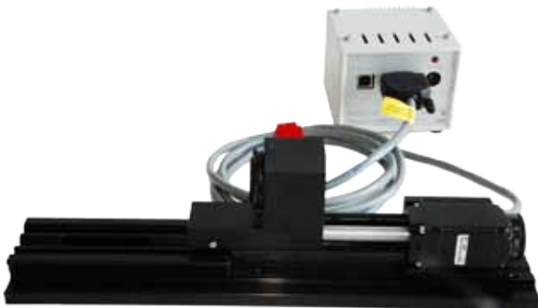
Fig. 72: Translation stage (TS) driven by a micro step motor (SM) carrying the triple reflector TR2
