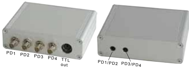
Fig. 62: Module N: Preamplifier PDA
