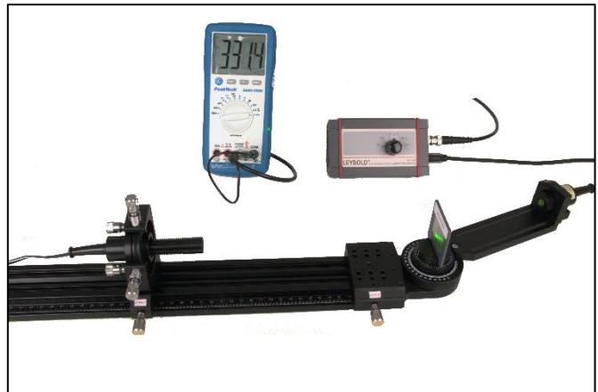
Fig. 4: Setup to measure the intensities of the grating maxima.
