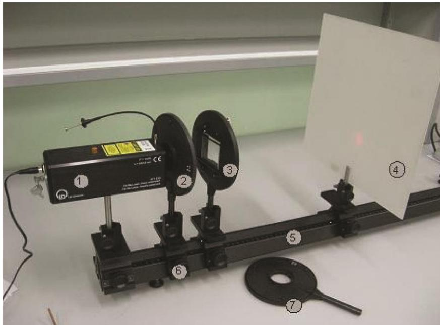
Fig.1. Experimental setup for observing interference phenomena created by means of Fresnel's biprism.
