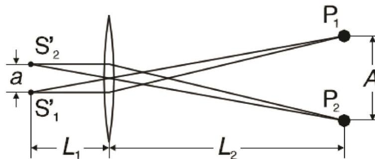
Fig.3. Determining the distance  $a$  between the virtual light sources.
