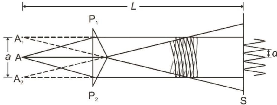
Fig.2. Schematic representation of the beam path at Fresnel's biprism.
