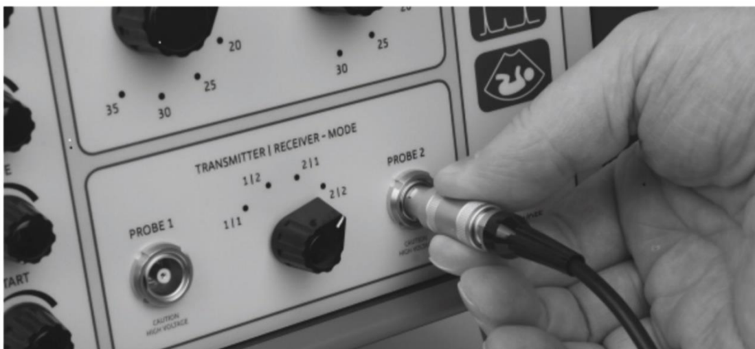
Figure 13. Connecting/disconnecting a transducer to GS200
