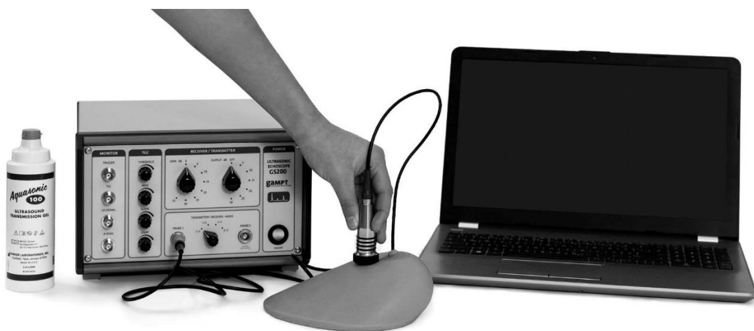
Figure 33. Laboratory setup for studying ultrasonic mammasonography
