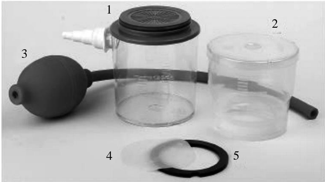
Figure 36. Heart model. Double container with rubber membrane for simulation of cardiac wall and heart valves movements: (1) lower container with tubing adapter, (2) upper container with lid, (3) rubber pressure ball with tubing, (4) membrane, (5) locking ring.
