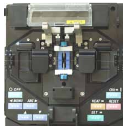
Fig. 27: Module F splicing device, interior view
