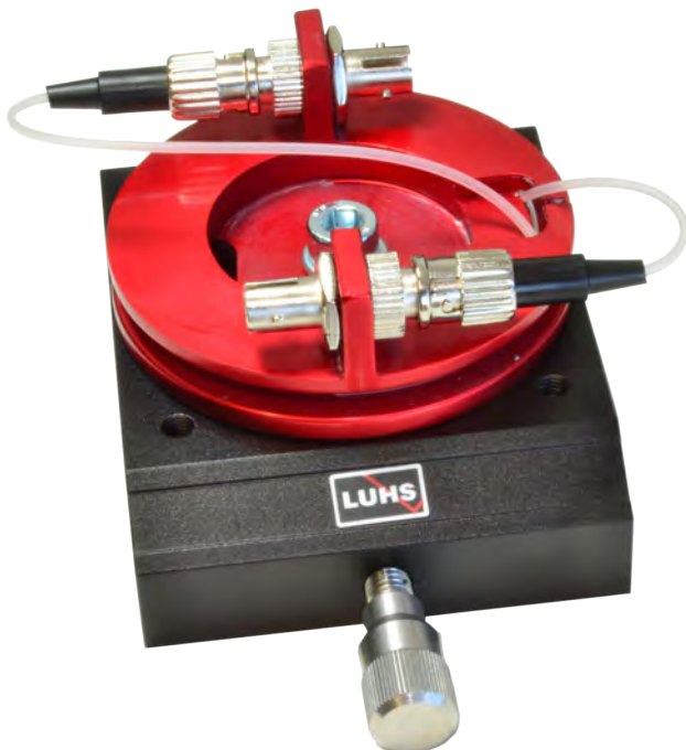
Fig. 35: Erbiem doped fibre 1.5 m
