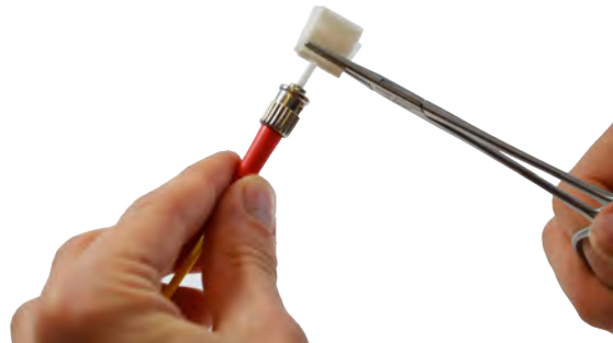
Fig. 48: Cleaning the front face of an optical fibre
