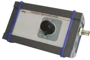
Fig. 43: Module P - Photodetector signal conditioning box
