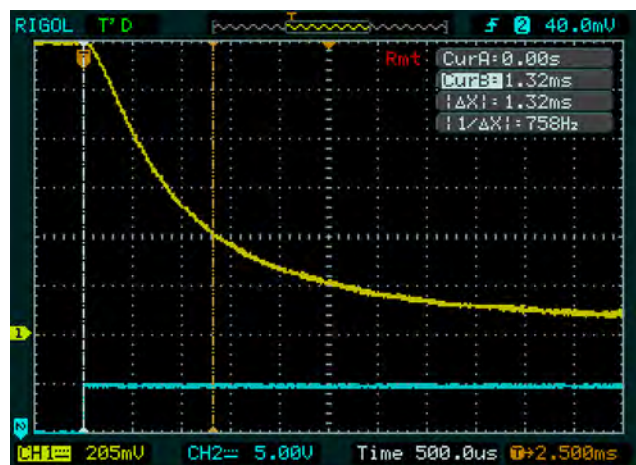
Fig. 53: Decay of fluorescence light
