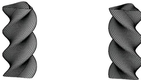
**Fig. 1.** A (non-optimized) pair of 3-start screw surfaces.
