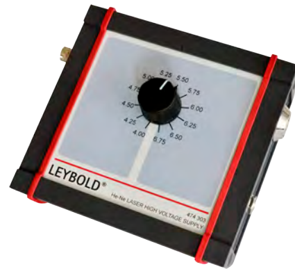
Fig. 26: High voltage power supply (6)
