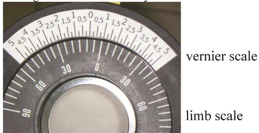
Fig.5. Vernier and limb scales of the analyzer.
