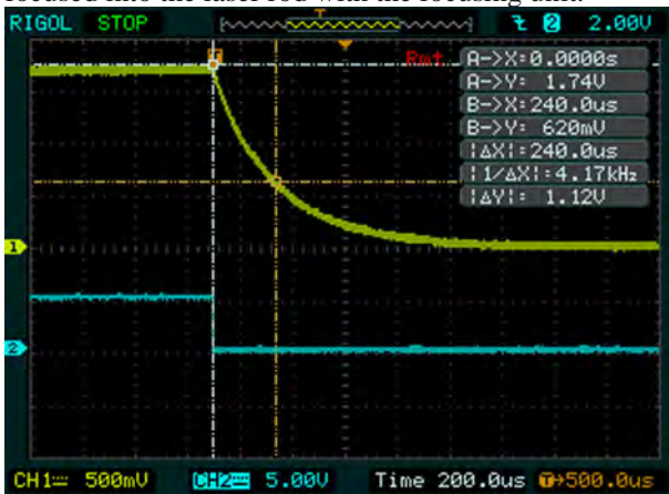
Fig. 6.4: Oscilloscope traces of pump power (upper) and detector G (lower)
