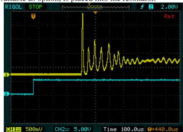
Fig. 6.7: The upper trace shows the photodetector signal and the lower one the injection current
