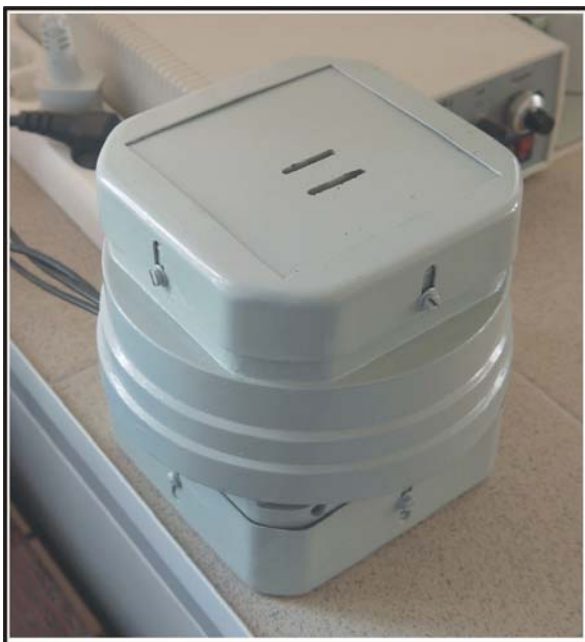
Figure 2. The cascade of Geiger counters, protected by a lead jacket.
