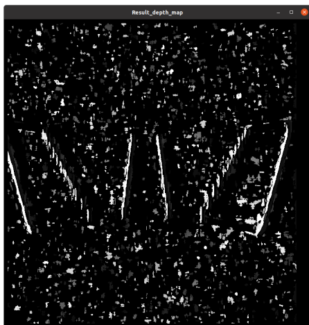
Fig. 11: Example of a poor depth map for stairs recognition system
