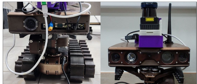
Fig. 4: Servosila Engineer's head. Left image: a monocular rear view camera. Right image (from left to right): a left monocular camera of a stereo vision pair, a flashlight, a camera with variable optical magnification, a right monocular camera of the stereo pair, on top is LIDAR.
