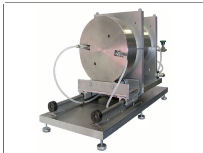
Figure 2. Custom built high pressure high temperature oven used for the pyrolysis of SiCN.
