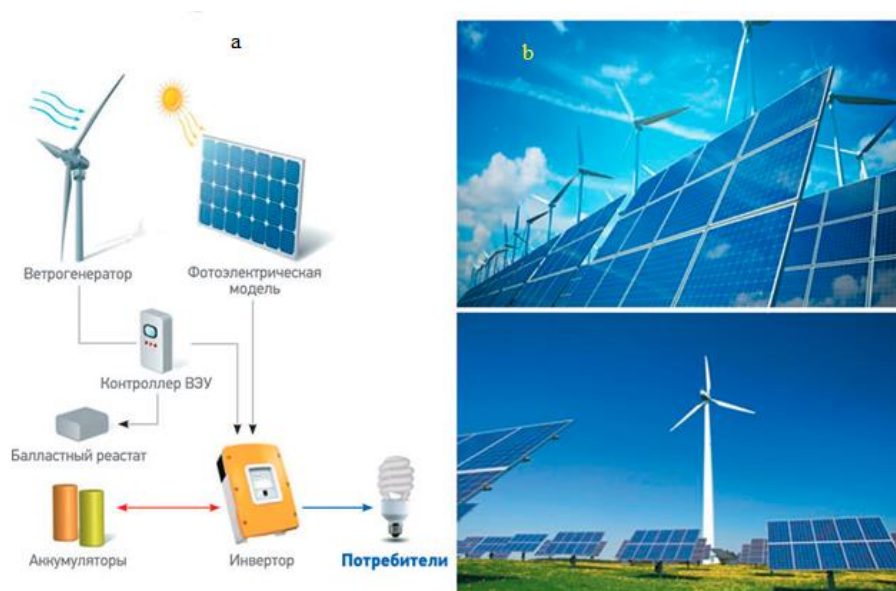
Picture 1 - Conditional scheme (a) and appearance (b) of a wind-solar power plant (wind turbine-wind power plant)
