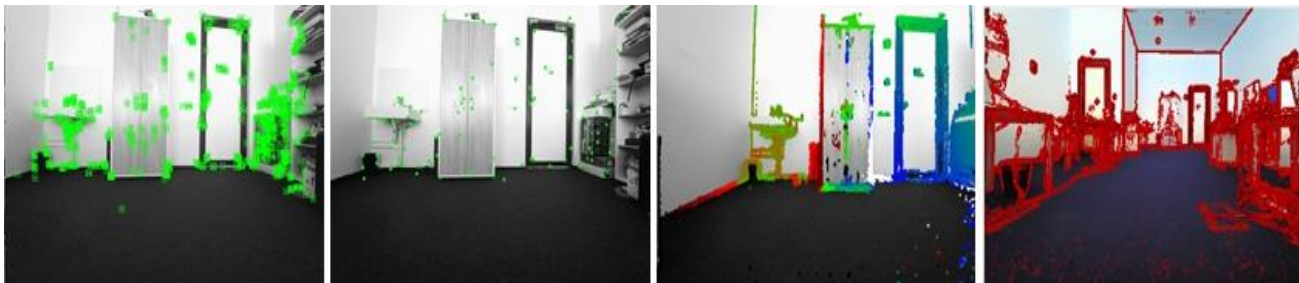
Figure 3. From left to right: Feature detection visualization by ORB-SLAM, REMODE, LSD-SLAM, and DPPTAM methods.
