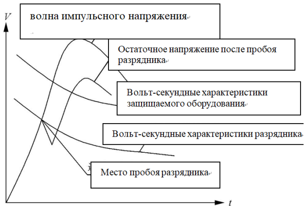
Figure 2. Coordination of insulation based on arrester protection
