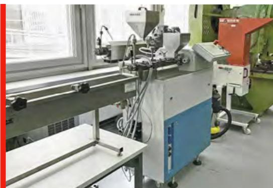
Fig. 1: Laboratory twin screw extruder
