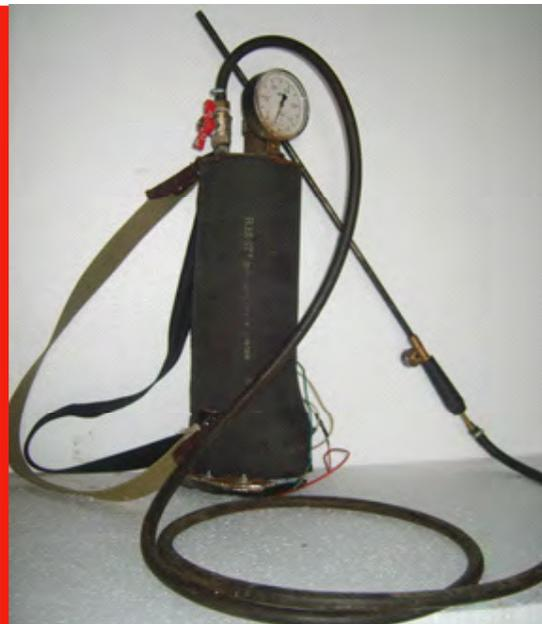
**Fig. 2: Electric steam generator.**
