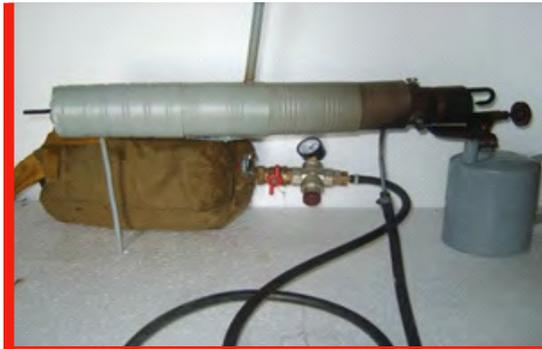
**Fig. 1: Autonomous steam generator.**
