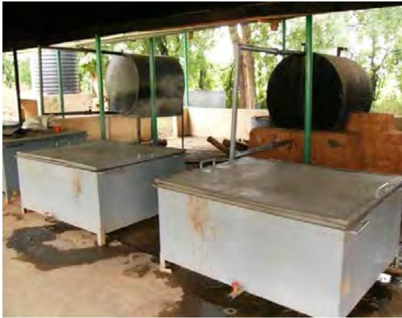
Plate 1. Old model parboiling system
