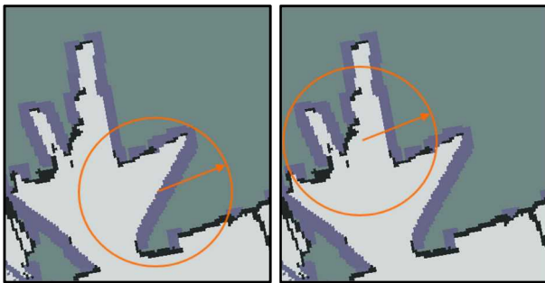
Fig. 5. A region of the original map. A preferred observing position by naive approach (left) and by the proposed approach (right). Circles and arrows show sensory radius of the robot.
