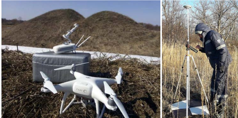
Figure 2. Quadcopter DJI Phantom 4 (left), special mark georeferencing by GNSS receiver (right).
