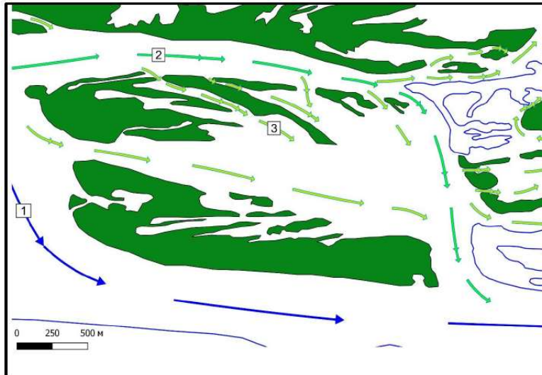
Fig. 4: The Types of Currents in the Studied Area (1 - Midstream, 2 - Subsidiary Flow, 3 - The Currents of the Inter-island Channels).
