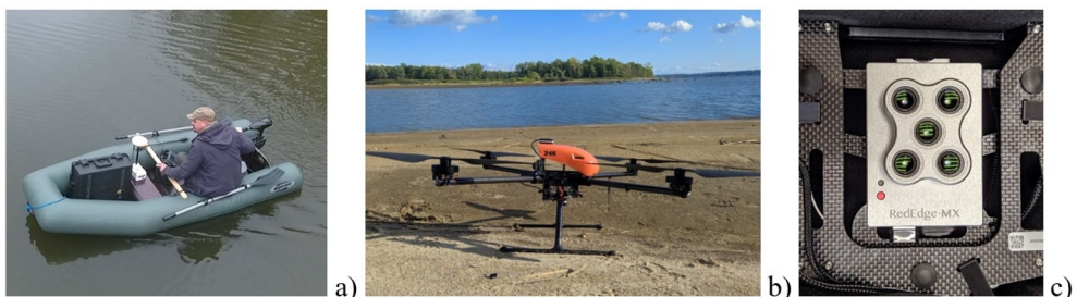
Fig. 1. Equipment used in the field surveys. Boat with Garmin GPS Map 178C chartplotter (a), Geoscan 401 Geodesy UAV (b), MicaSense RedEdge-MX camera (c).
