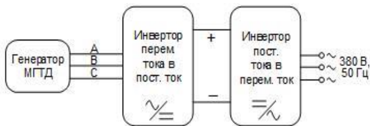
Figure 1 – Functional diagram of power electronic converter
