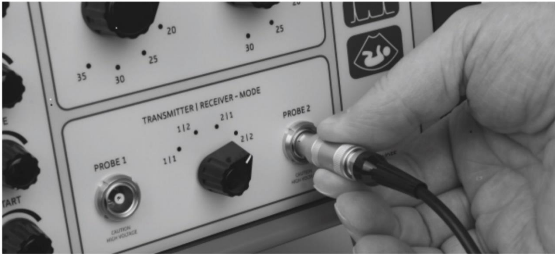
Figure 13. Connecting/disconnecting a transducer to GS200
