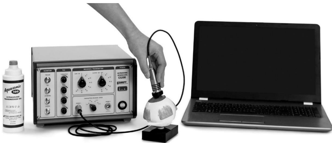
Figure 27. Measurement of times of flight in an eye phantom as an example of the biometric ultrasonic application
