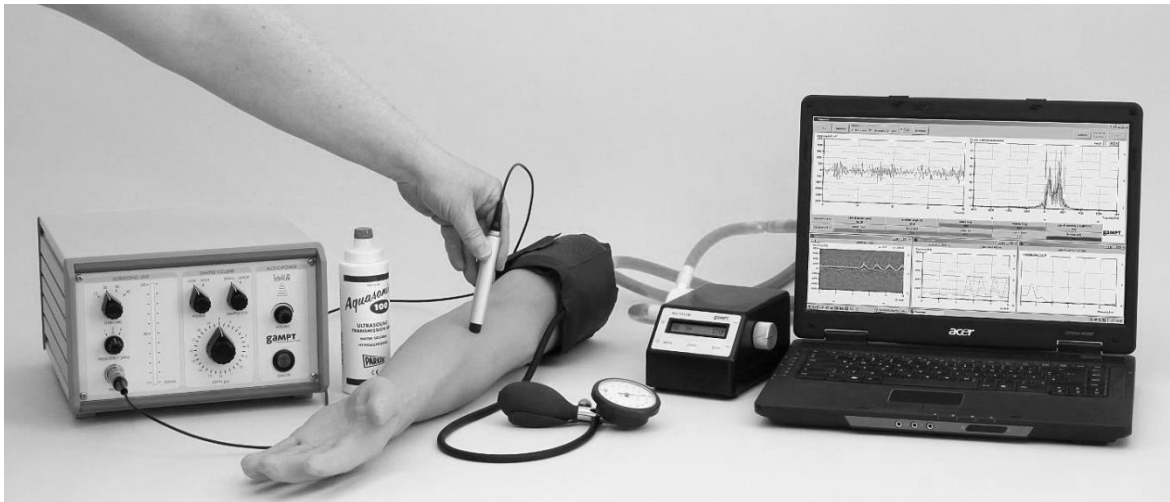
Figure 47. Laboratory setup for studying ultrasonic sonography
