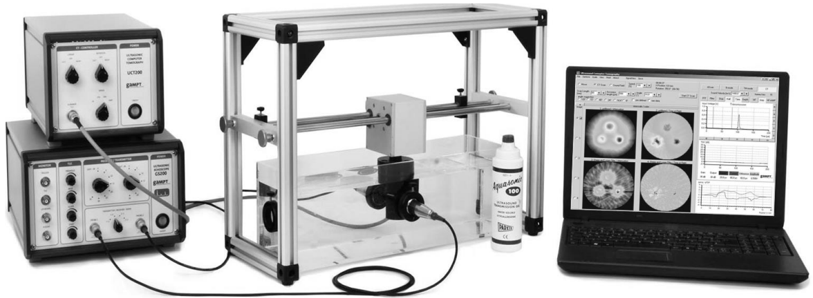
Figure 55. Experimental setup for performing ultrasonic computed tomography
