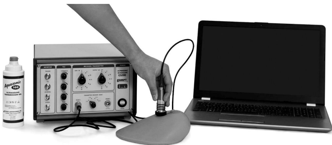
Figure 33. Laboratory setup for studying ultrasonic mammasonography
