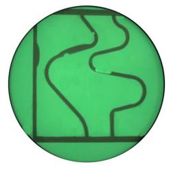
Fig. 1: Picture of a model blood vessel with a contrast medium on a fluorescent screen, taken with a digital camera.
