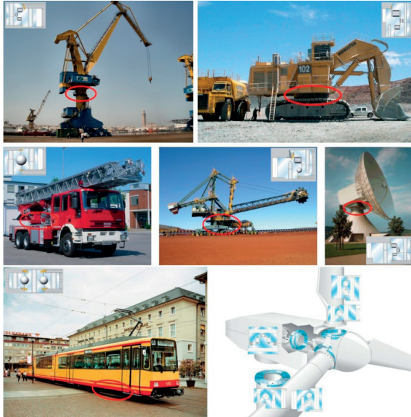
Figure 1 Examples of the slewing bearings applications
