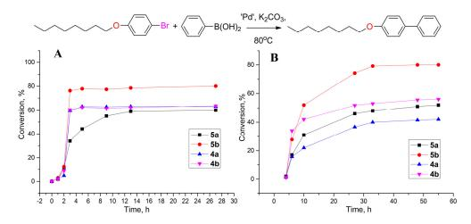
**Figure 4.** Conversion of *p*-octyloxybrombenzene vs. time in Suzuki–Miyaura reaction between *p*-octyloxybrombenzene and phenylboronic acid in DMF (**A**) or DMF:water 1:3 mixture (**B**).  $n(p-C_8H_{17}OC_6H_4Br) = 0.16 \text{ mmol}$ ,  $n(PhB(OH)_2) = 0.28 \text{ mmol}$ ,  $n(K_2CO_3) = 0.28 \text{ mmol}$ ,  $n(4a,b \text{ and } 5a,b) = 0.16 \mu \text{mol}$ ,  $80 \text{ }^\circ\text{C}$ , and V = 0.8 mL.
