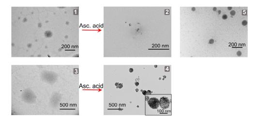
**Figure 3.** TEM images of **4a** before (1) and after (2) treating with ascorbic acid; **4b** before (3) and after (4) treating with ascorbic acid, and  $3b+K_2PdCl_4$  (5) treated with ascorbic acid, with different scale bars.
