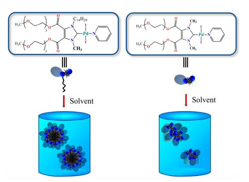
**Scheme 4.** Schematic representation of aggregates formed by systems **4a** and **b** with different lipophilicity.
