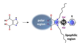
Scheme 1. Metallosurfactant on a 1H-imidazole-4,5-dicarboxylic acid platform.
