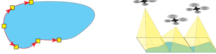
Fig. 1. Illustration of caging a flood area by multiple UAVs.
