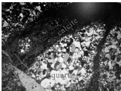
Fig. 7. A microscopic photograph of limestone containing chert (under orthogonal light; magnification: 5×10)
