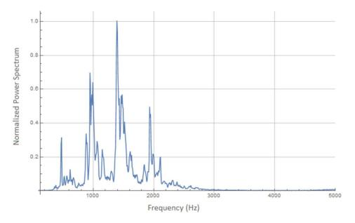
Fig. 1. Typical energy spectrum of engine noise. The crankshaft frequency is 20 Hz (1200 RPM).
