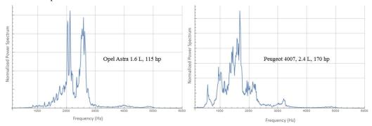
Fig. 4. Spectrums of acoustic noise at different engine volumes.
