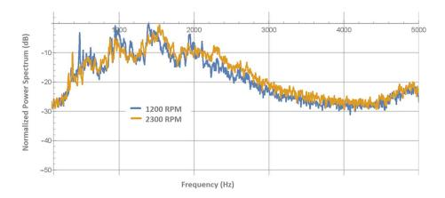
Fig. 2. Energy spectrums with a change in the frequency of rotation of the crankshaft.
