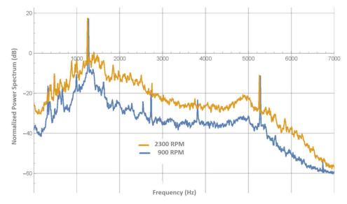
Fig. 3. The dependence of the power level on the frequency of rotation of the crankshaft.
