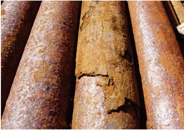
Fig. 1.6. External corrosion of casings
