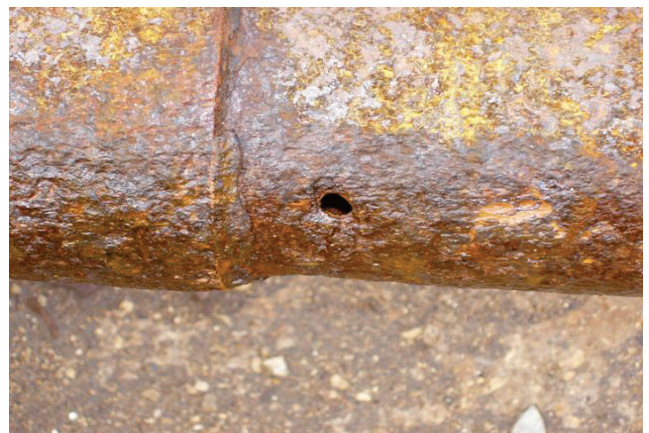
Fig. 1.7. A penetration near the socket plus external corrosion
