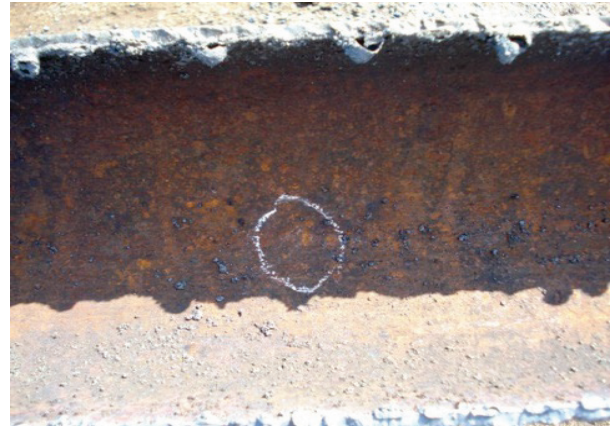
Fig. 1.8. Internal corrosion spots
