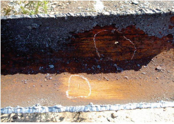
Fig. 1.8. Internal corrosion spots
