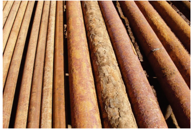
Fig. 1.6. External corrosion of casings
