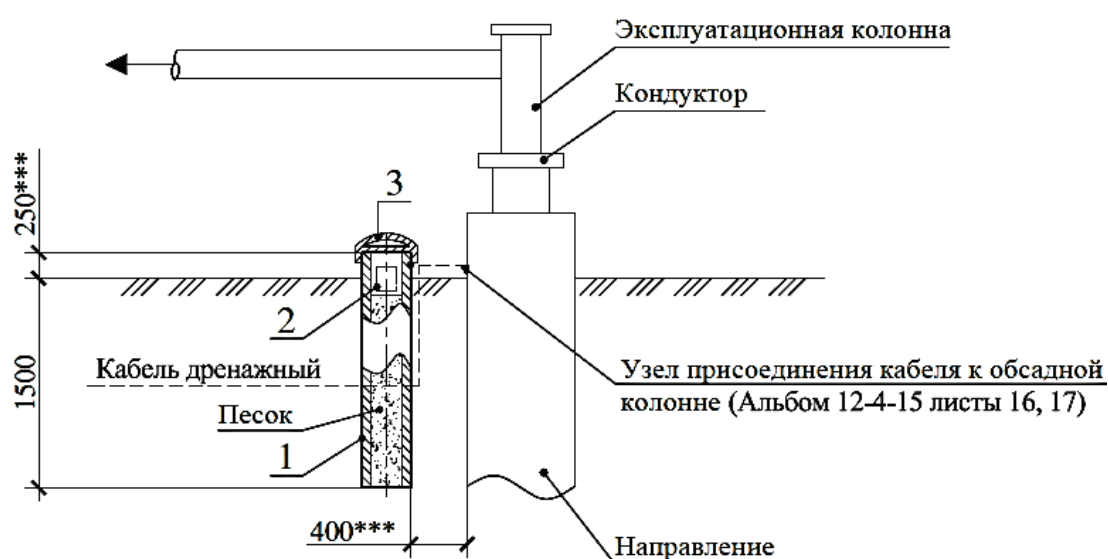
Fig. 4.4. Potential measuring pit: 1 – PE80 pipe; 2 – Copper-sulfate electrode; 3 – Cap
