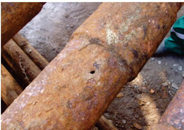
Fig. 1.7. A penetration near the socket plus external corrosion
