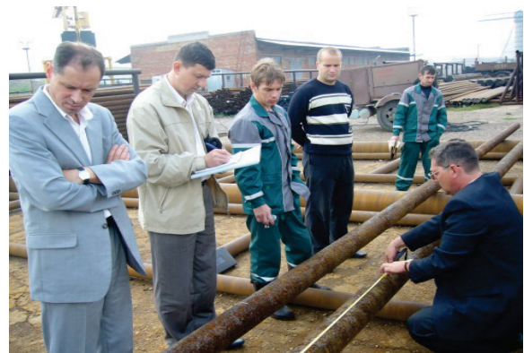
Fig. 1.27. Visual inspection of casings
