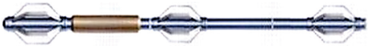
Fig. 7.11. Multifrequency electromagnetic thickness measurer METT
