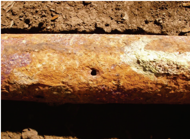
Fig. 1.9. External penetrating corrosion of casings
