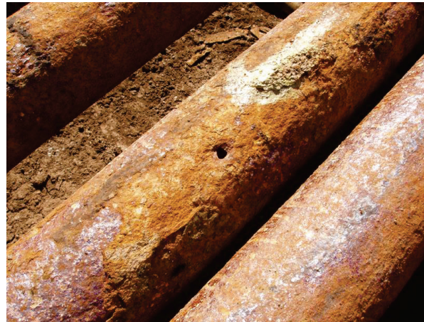
Fig. 1.9. External penetrating corrosion of casings
