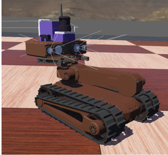
Fig. 4. The final simulation model of the Servosila Engineer robot in Webots.
