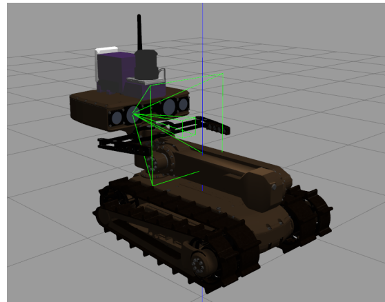
Fig. 2. Gazebo simulation model for Servosila Engineer
