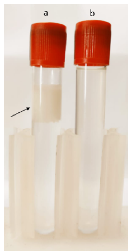
Figure 13. Visual appearance of surfactant solutions with the concentration of 30% NaCl at (a) 20 °C for SA-3 and (b) 200 °C for Vector.
