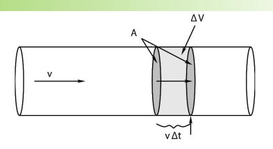
In figure we see fluid flowing from left to right in a circular pipe. The pipe is assumed to be "frictionless" for the time being – to exert no drag force on the fluid flowing within – and hence all of the fluid is moving *uniformly* (at the same speed v with no relative *internal* motion) in a state of *dynamic equilibrium*.
