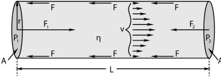
In figure a circular pipe is carrying a fluid with viscosity  $\mu$  from left to right *at a constant speed*. Once again, this is a sort of dynamic equilibrium; the net force on the fluid in the pipe segment shown must be zero for the speed of the fluid through it to be maintained unabated during the flow.
