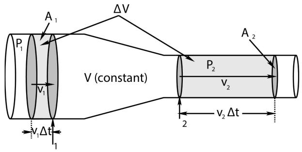
Figure shows a fluid as it flows from just such a wider pipe down a gently sloping neck into a narrower one. As before, we will ignore drag forces and assume that the flow is as uniform as possible. The pressure, speed of the (presumed incompressible) fluid, and cross sectional area for either pipe are  $P_1$ ,  $v_1$ , and  $A_1$  in the wider one and  $P_2$ ,  $v_2$ , and  $A_2$  in the narrower one.
