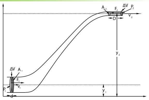
A circular cross-sectional necked pipe is arranged so that the pipe *changes height* between the larger and smaller sections. We will assume that both pipe segments are narrow compared to the height change, so that we don't have to account for a potential energy difference (per unit volume) between water flowing at the top of a pipe compared to the bottom, but for ease of viewing we do not draw the *picture* that way.
