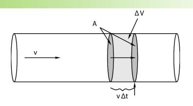
In a time  $\Delta t$ , all of the water within a distance  $v\Delta t$  to the left of the second shaded surface will pass *through* this surface and hence past the point indicated by the arrow underneath. The volume of this fluid is just the area of the surface times the height of the cylinder of water:
