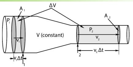
In a time  $\Delta t$  a volume of fluid  $\Delta V = A_1 v_1 \Delta t$  passes through the surface/past the point 1 marked with an arrow in the figure. In the volume between this surface and the next grey surface at the point 2 marked with an arrow *no fluid can build up* so actual quantity of mass in this volume must be a *constant*.
